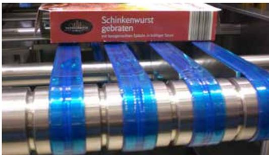
T-profiles are a very good solution to convey different light-weight goods and food product. On such conveyors there are usually several T-profile belts installed parallel to each other. The V-guide on the running side ensures a straight and precise movement. BEHAbelt offers T-profiles in various geometries, shore-hardness and color combinations.
