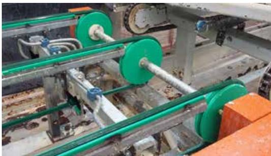
Ridge-top-V-belts by BEHAbelt are made of weldable PU or TPE. They are specially suitable for demanding conveyor applications in tile processing and production of construction materials. This product range is made of durable compounds in different shore-hardness-grades.
